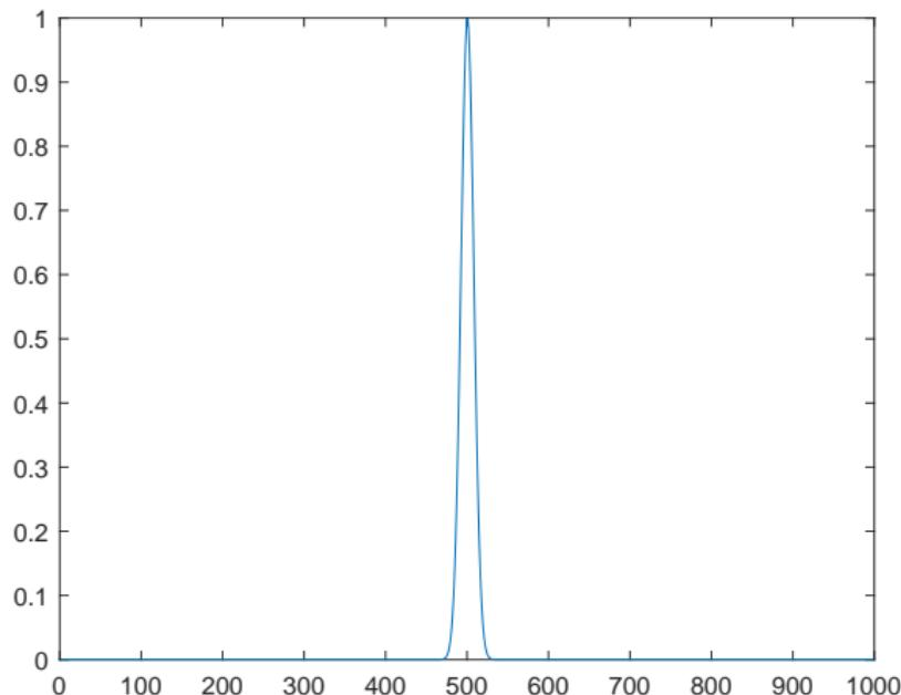
Figure: Low-pass filter – gaussian  $e^{-a\xi^2}$
