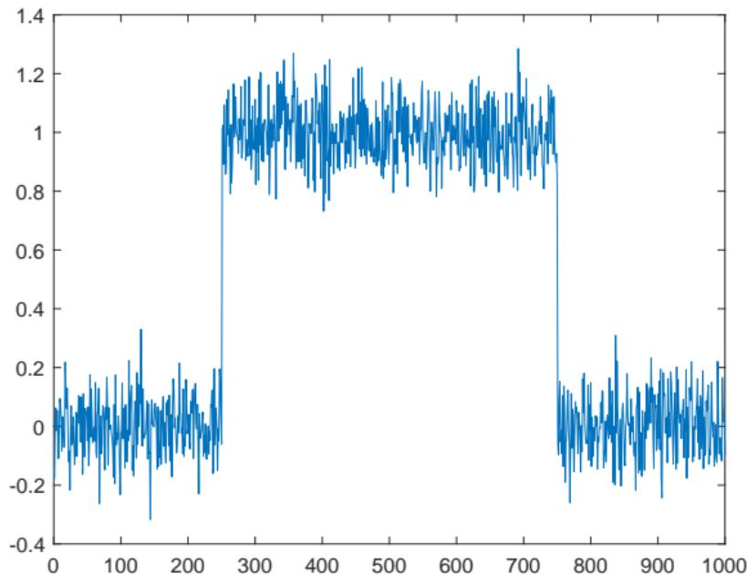
Figure: Rectangular signal with noise
